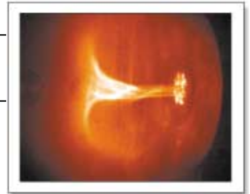
Spheromak initiation using planar magnetized plasma source.
